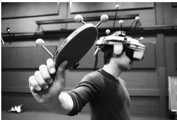
Figure 3. Photograph of a participant holding the paddle and wearing the HMD. Participants had to hit the virtual table tennis balls seen as a stereoscopic image within the HMD. The motion trajectory of the paddle was recorded and analyzed.
