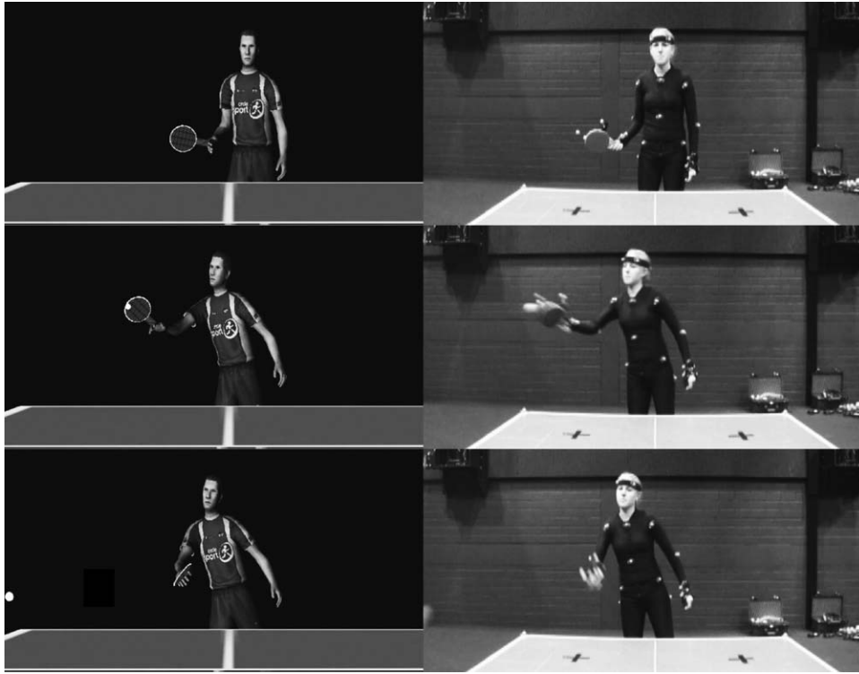
Figure 2. A visualization of three frames of one of the 12 different table tennis stroke animations. The animations (left) were created by using motion capture data from an actor performing table tennis strokes (right). All 12 strokes were motion captured using a VICON motion capture system with 16 infrared cameras. The cameras recorded 46 (24 for upper body and 22 for lower body) infrared markers that were attached to the body of the actor, five markers that were attached to the paddle, and the table tennis ball, which was coated with infrared reflective paint.
